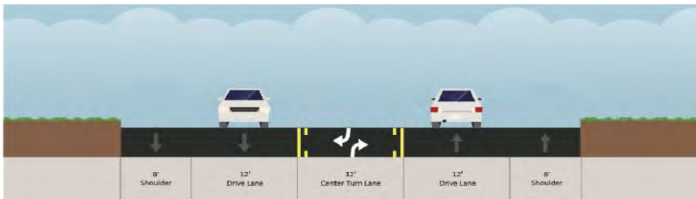
Figure 2-9 Cross-Section of SR 4 Showing Planned SHOPP Project
